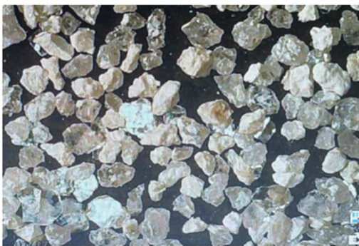
Washed sand 600 micron. High sphericity; sub angular
