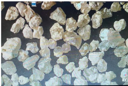
Washed sand +1.18 mm. High sphericity; sub angular-sub rounded
